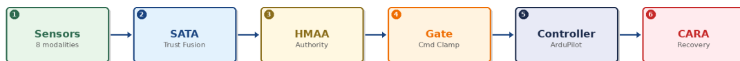
Figure 2. Authority-governed flight pipeline: sensor data flows through SATA trust fusion, HMAA authority computation, command gating, and ArduPilot execution, with CARA recovery enforcement.
