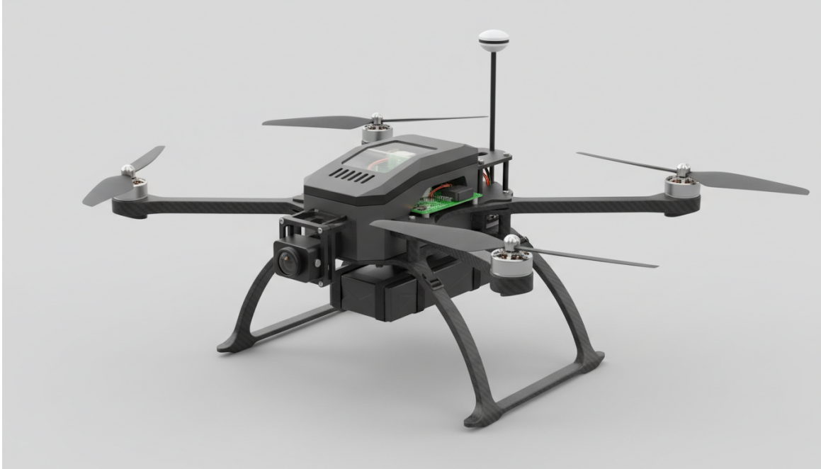
Figure 1. HMAA-UAV platform: 500mm carbon fiber quadcopter with Cube Orange+ autopilot, Jetson Orin NX companion, Livox Mid-360 LiDAR, dual GPS, thermal camera, and multi-sensor array.
